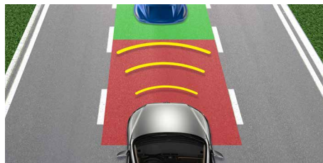
Forward Collision Warning System (FCWS) helps maintain a safe distance
