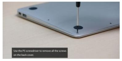
Use the P5 screwdriver to remove all the screws on the back cover.
