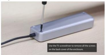
Use the T5 screwdriver to remove all the screws on the back cover of the enclosure.
