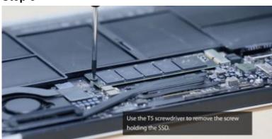
Use the T5 screwdriver to remove the screw holding the SSD.
