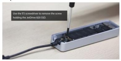
Use the T5 screwdriver to remove the screw holding the JetDrive SSD.
